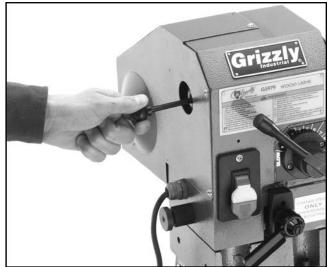
Figure 9. Removing the spur center.
